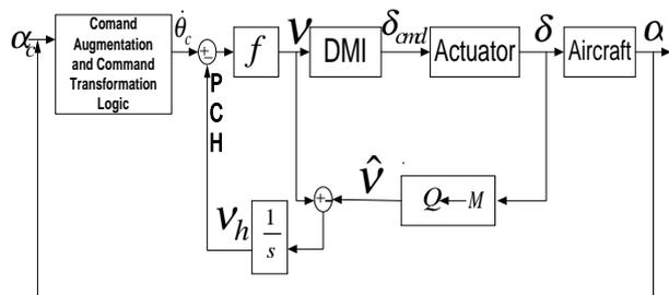
Fig. 5. DMI based  $\alpha$ -CAS with PCH compensation.
