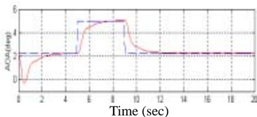
Fig. 7. Compensation of PCH for slow actuator.
