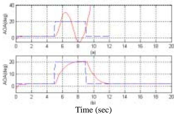
Fig. 8. Effect of PCH in case of actuator saturation.
