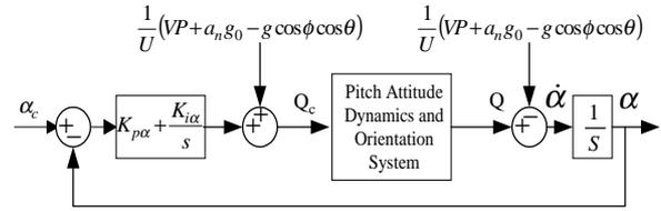
Fig. 2. Outer-loop of  $\alpha$ -CAS for stability analysis.
