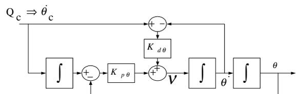
Fig. 4. Pitch orientation pseudo control loop.
